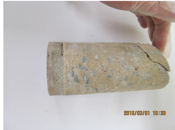
Figure 9: Core 5 Beneath splash zone was in the tiled area above the first horizontal reinforcement steel on the east side of the pool. A tile and intermediate layer is observed over concrete with blue aggregates and a different type of cement.
