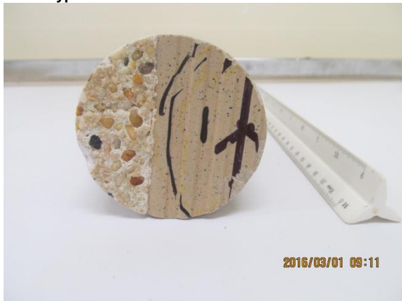
Figure 12: Core 1 Splash zone sample showing the tile and stone topping over the core.
