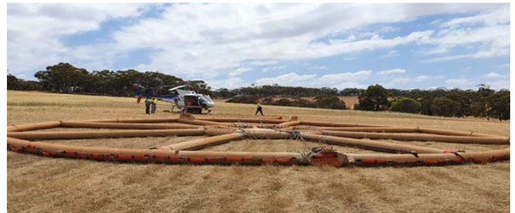
Airborne geophysical surveys may comprise of magnetic, radiometric, gravity, or electromagnetic surveys. Above is an image of the measurement apparatus which is used
