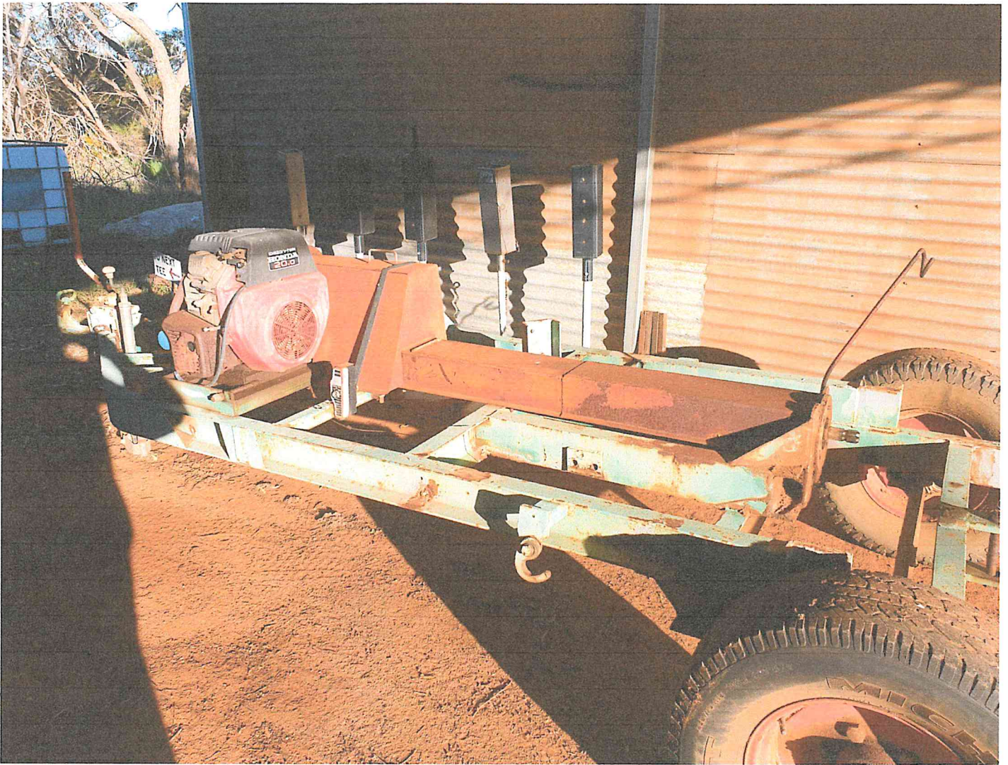
OUR CURRENT POWER SOURCE FOR OUR MOWER, 20HP HONDA MOTOR DRIVING A PTO SHAFT.
